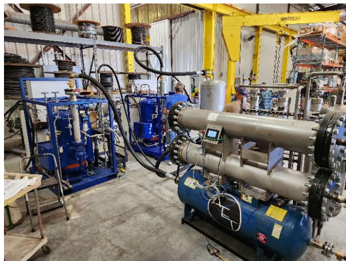
Figure 5. Shown is the AET membrane skid test setup. The membrane skid is shown connected to two rotary screw helium compressors.
