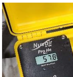
Figure 6. The handheld gas analyzer is shown connected to the second stage membrane permeate stream. At the time this photo was taken, the permeate stream had reached 57.8% purity. Due to manual operation and transient pressure/flow fluctuations, helium concentrations at this point varied significantly, with real-time readings occasionally exceeding 60%.
