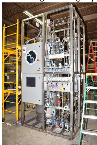
Figure 4. Shown is the AET HP series purifier built for processing gas mixtures at a hypersonic wind tunnel facility. This HP series was designed to receive 85% He/15% N 2 mixtures and purify to at least 99.9% (3.0 grade). Based on design enhancements to the adsorption circuits and liquid air separator, the system was anticipated to handle lower inlet helium concentrations while maintaining comparable outlet purity.
